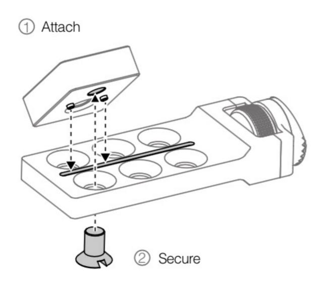
Check that the Mounting Adapter is secure before attaching your accessory.
