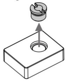
Attach the Mounting Adapter to the Universal Mount. Align the studs with the narrow slot, and then secure the Mounting Adapter with the 1/4" screw on the Universal Mount.
