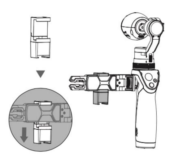
Mount your equipment on one of the cold shoe mounts. The bottom cold shoe mount rotates 360 degrees.
